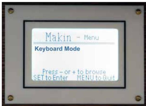
Allows the keyboard sensitivity to be adjusted.
