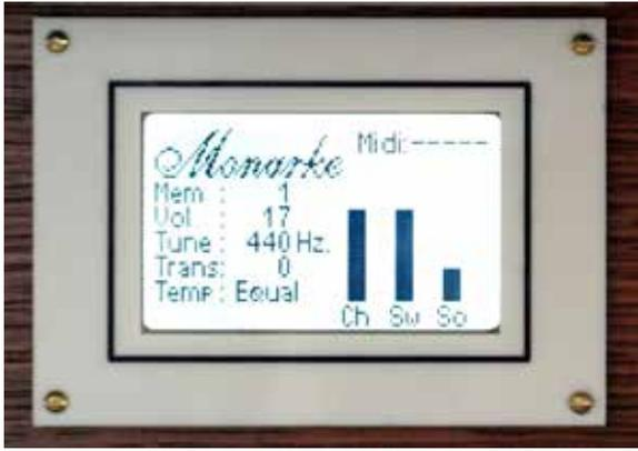
The function of the display is to show various settings of the instrument and to allow the settings to be programmed. The display Shows:-
