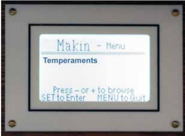
Allows the selection of Temperaments. The default setting is Equal.
