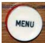
The Menu piston is used for displaying the menu on the LCD display.
