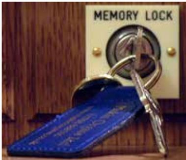
The Memory Lock (shown in the off position) is used to store personal registrations, volume, tune, transposer settings, MIDI-stop settings and Menu settings. The memory has to be “opened” by turning the memory lock key to allow changes to be stored in the instruments memory.
