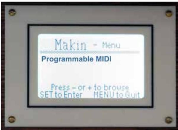
Allows the keyboards to be assigned to MIDI channels and patches (Voices) in combination with the MIDI stop or piston associated with the keyboard. With the programmable MIDI stops, you can control any module voice (1-128) through any MIDI channel (1- 16).
