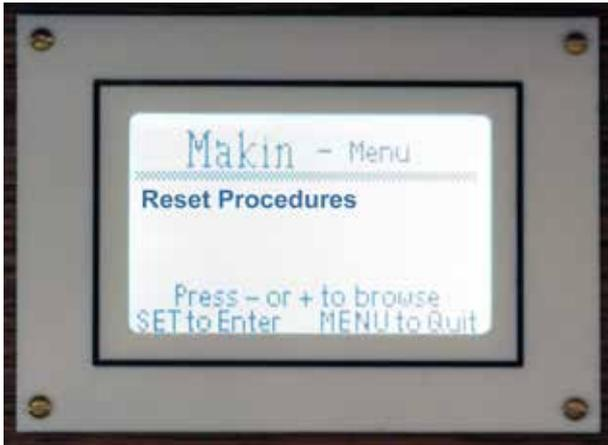
Allows the capture system to be reset to Factory default settings.
