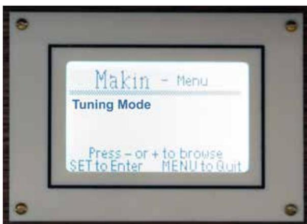
Allows the adjustment of the frequency setting of the instrument by stepping up or down with the + or - pistons. The default setting is 440 Hz corresponding to A in the same octave as middle C. The range is 426 Hz to 454 Hz in steps of 1 Hz allowing up to a quarter note change in each direction.
