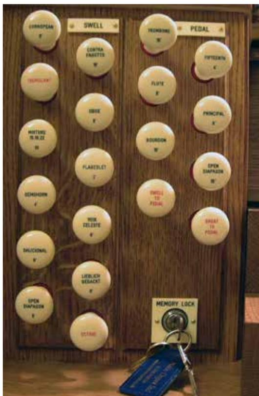
A Drawstop can be turned on (activated) by pulling a stop knob out. A stop can be turned off (deactivated) by pushing in a stop. The position of a stop shows if a stop is activated or deactivated. On British instruments the draw stops of the Swell are located on the left of the keyboards and the stops of the Great on the right. Drawstop columns are offset vertically to maximize the space surrounding the stop which allows easier access.
