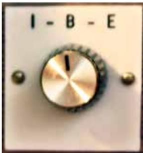
Some instruments have a three position switch which allows switching between internal (I) speakers, external (E) speakers and having both internal & external (B) speakers. Other instruments have their own internal speaker system or will have an external loudspeaker system. At the rear of the instrument (or possibly mounted internally) are connectors (octal sockets) that can be connected with a special cable to an external loudspeaker system.
