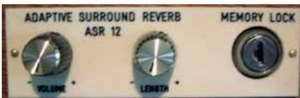
With the rotary control the volume and length of this acoustic effect can be adjusted continuously.
