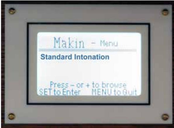
This enables the Intonation to be set so that when the instrument is switched on the intonation set in memory (default) will be selected.
