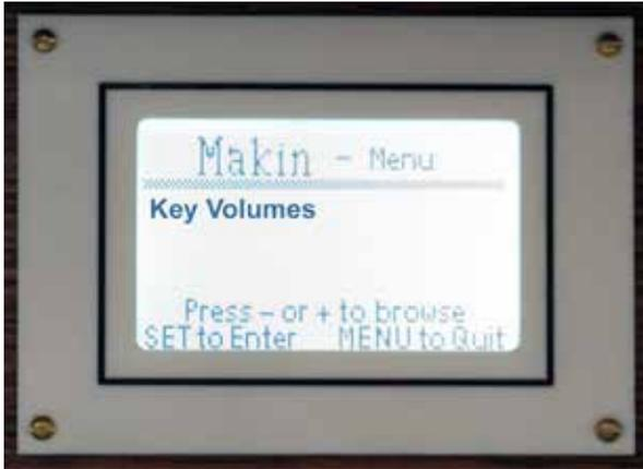
Allows the setting of volume for individual keys per stop and intonation. The function consists of the following sub-functions:-
