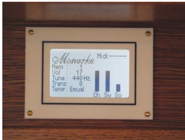
This graphical display shows many functions including the memory in use, volume, tuning, pitch, transposition, temperament and the position of the swell boxes
